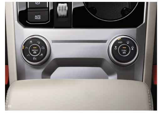
01 Air suspension ensures you enjoy ultimate driving comfort on every trip, adapting the height of the car to the terrain, with a choice of Normal, Comfort, Off-road and Special Off-road driving profiles.02 Thanks to rear-axle steering, cornering on twisty roads and parking on city streets is a whole lot easier in the Touareg.
