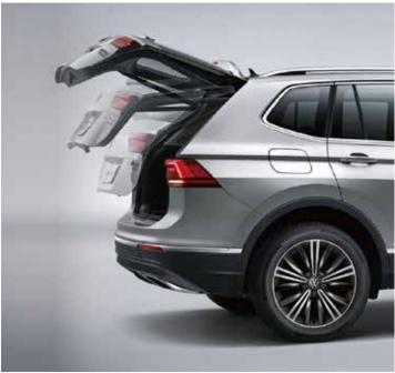
A sensor controlled electric tailgate system that opens and closes the tailgate with a sweep of your foot.
