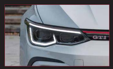
The GTI features full LED headlights with cornering function and all weather lights, as well as an illuminated strip between the headlights.
