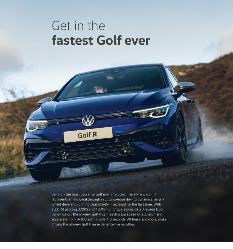
The all-new Golf R's 4MOTION All-Wheel Drive system introduces rear-axle torque vectoring, delivering a whole new level of performance. While cornering, more power can be directed to the wheel on the outside of the curve in a matter of milliseconds, therefore significantly increasing the agility of the Golf R, and your driving pleasure.
