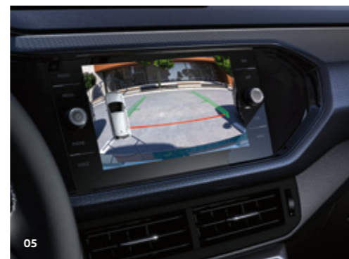
05 The Rear View reversing camera helps in reversing manoeuvres. 1) The camera image on the radio display or navigation system shows the area behind the vehicle. OE
