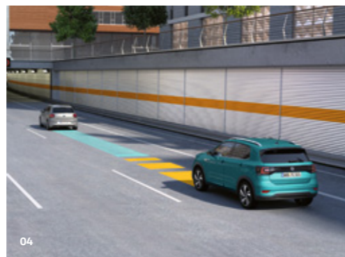
04 The ACC adaptive cruise control can help you to maintain a set top speed 3) and fixed distance from the vehicle in front. 1) OE
