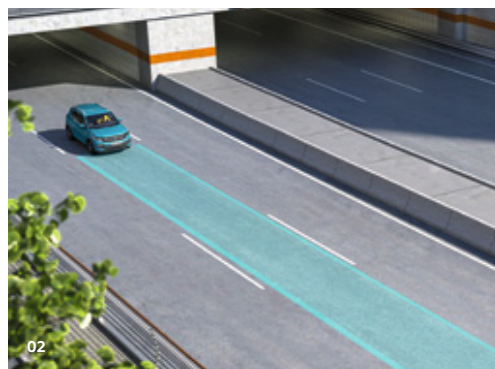
02 The Lane Assist lane departure warning system can detect – from speeds of 60 km/h – whether the vehicle is unintentionally leaving its lane. 1) The corrective steering assistance feature prompts the driver to return their attention to the road. 1), 2) S
