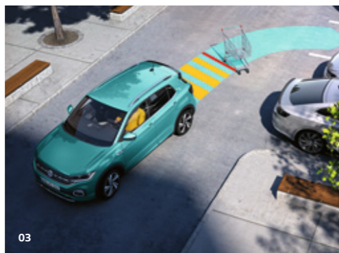
03 When manoeuvring, the Park Distance Control system issues acoustic and visual warnings when it detects obstacles in front of or behind the vehicle. 1) The integrated manoeuvre braking function can prevent collisions, or minimise their impact, by applying an emergency brake when reversing at speeds up to 10 km/h. 1) You can activate the manoeuvre braking function at the touch of a button, enabling it to intervene when the vehicle is driving forward as well. LF ST
