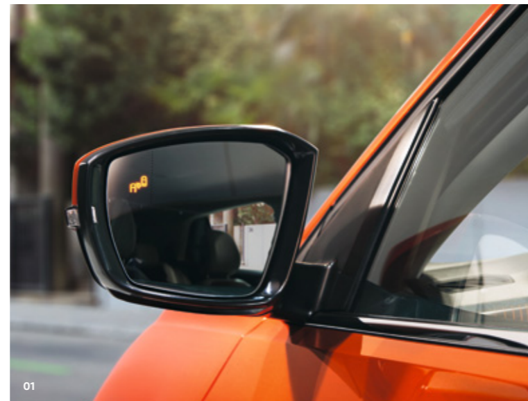
01 The Blind Spot sensor activates LEDs in the relevant exterior mirror to warn you if there is a vehicle in your blind spot. 1) When reversing out of a parking space, the integrated Rear Traffic Alert system can monitor the area behind your vehicle and warn you of any traffic that crosses this space. 1) OE
